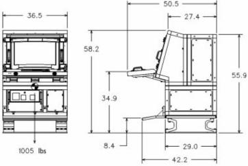
The illustration shows dimensional data for the Grade A sit-down version of the LSTD-R console. Also available is a stand-up version that increases the height of the system by five inches. All dimensions are listed in inches.
